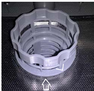
Poorly secured filter
