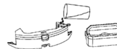
Electrically operated water tank
